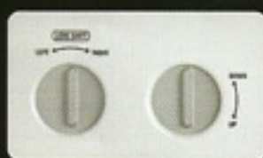
The Lens Shift Dial (Right Left, Up/Down) on the top side of the projector.
